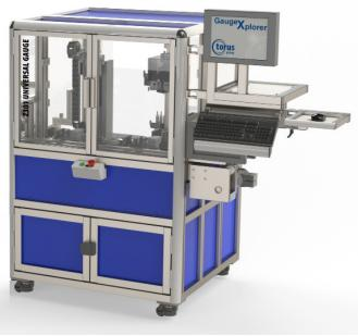
The Universal Trimmed & Finished Can Inspection Gauge from Torus Measurement Systems defines the standard for dimensional of beverage/beer cans.
