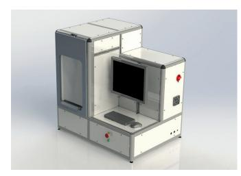
The B303 Semi-Automatic Bottle Burst Gauge has been developed to verify production containers meet the minimum pressure requirements.
