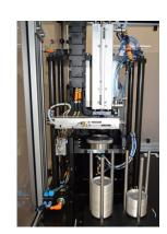
The new Z605 model offers our customers the ability to perform both end buckle and burst tests without the need for change parts.
