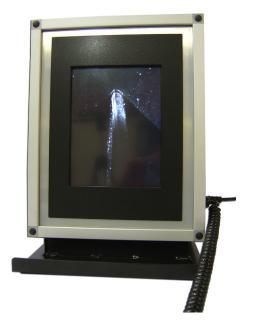
Fan blade edge condition is a significant factor in the thrust performance of an engine. Torus' Edge Profile Inspection System is a low cost optical instrument designed for the visual inspection of the leading and trailing edges of turbine edge fan.
