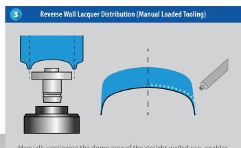
Manually sectioning the dome area of the straight walled can, enables the operator to collect complete dome profile and reverse wall lacquer distribution analysis.
