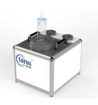
Designed specifically for 2 piece can manufacturers who "reform" their cans, this small inspection gauge gives critical measurement information on the setup of each head of your reformer.
