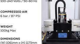
The Z308 Dome Growth/Reversal Gauge provides detailed information about the overall change in length of the can when pressure is applied and subsequently removed.
