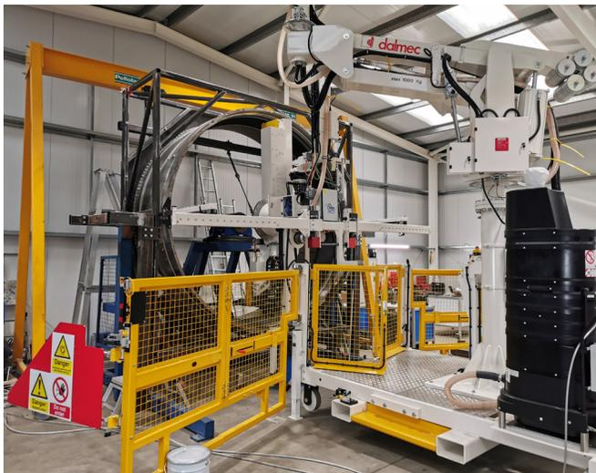
**With the ever increasing need for Turbo Fan engine efficiency in mind, Torus Group developed the A521 CNC Fan Track Boring machine. The machine produces an accurate fan track bore in a fraction of the time of any other system whilst at the same time requires fewer personnel for set-up and operation.**
